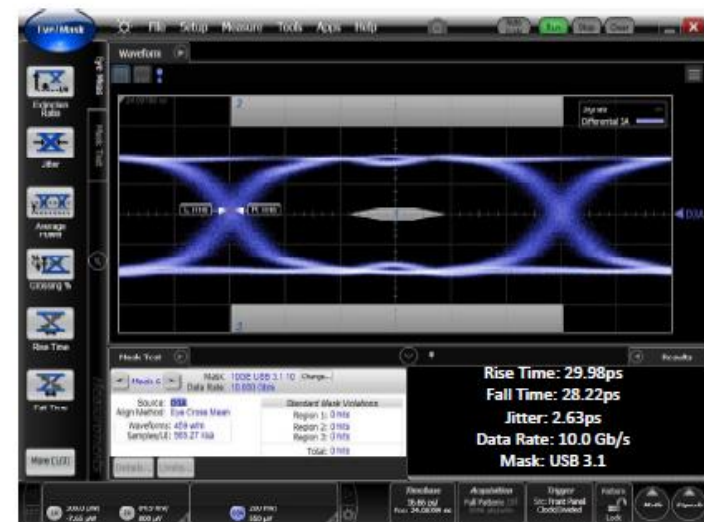
10Gb/s (USB 3.1) Eye Diagram without RClamp3361ZA
